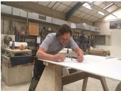
At Gloucester, all our setting-out drawings are produced on plywood that has been painted white. Using squares, straight-edges, rulers, compasses and pencils I set about constructing the drawing of the profile. Once completed I then made couple of templates of the profile which I then took to site and held them against the stone to see how well they matched up. Not bad, but to not quite right.
